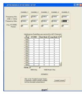
This screen is used to setup the interference messages from channels 1-5.
